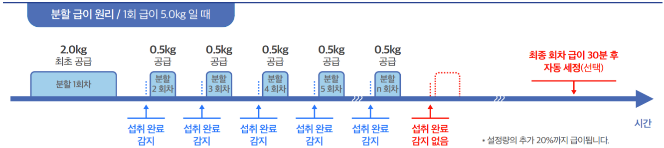
Figure 1. Feeding principles of automatic feeders for lactating sows. The figure was provided by M3SEN and is reproduced with permission.
