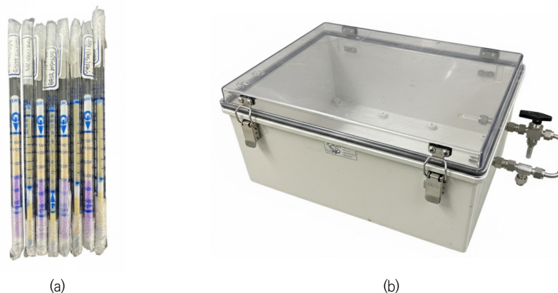
Fig. 3. Picture of ammonia detector tube and vacuum box used in this study. (a) The measuring range of the detector tube (GASTEC) was 5-100 ppm, and when the concentration exceeded this range, a 50-500 ppm detector tube was used; (b) Vacuum box (21.6 L).
